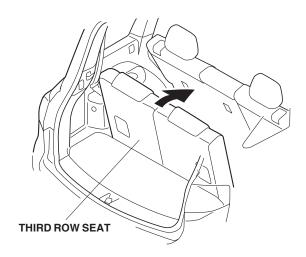
3. Using a small flat-tip screwdriver, remove the right and left rear side panel covers by releasing the retaining tab. Save the covers so they can be reinstalled when the cargo cover is removed.
