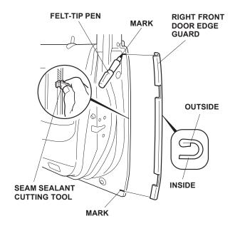
5. Position the cutting edge of the seam sealant cutting tool against the door edge, and trim the seam sealant between the marks at the top and bottom of the door edge.
