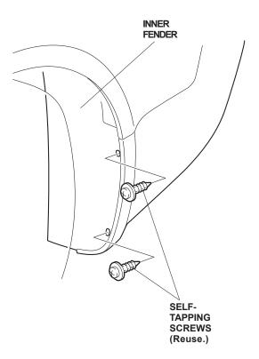
Position the left bracket on the inner fender, and reinstall the two self-tapping screws.
