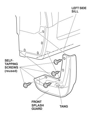
4. Turn the steering all the way clockwise and repeat step 2 and 3 to install the right front splash guard.
