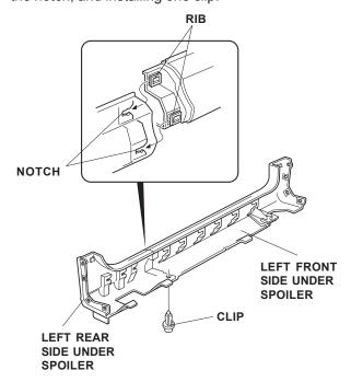
10. Slide the nine clips (removed in step 8) into the holders on the new side under spoiler through the slots, and align the tabs on the clips with the cutouts on the holders. Remove the existing rubber spacers from the clips, and install a new rubber spacer onto each of the nine clips.
