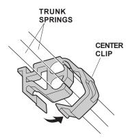
11. With an assistant holding the trunk lid open, remove the old trunk springs from the trunk hinge arms using the special tool. Wear heavy gloves to protect your hands, and pull the special tool slowly and carefully toward you.
