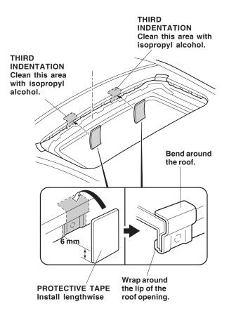
Install the protective tapes at the third indentations in from each side of the moonroof opening. Remove the adhesive backing from the protective tape and attach one at each position. Wrap 6 mm of protective tape around the lip of the moonroof opening. 9. Place the two front brackets and two side brackets into position over the protective tape and around the lip of the roof opening, and tape them into position with a piece of masking tape.
