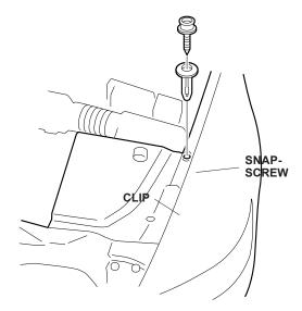
6. Pull the mask toward the left fender, and slip the left pocket of the bumper section onto the left front corner of the fender.
