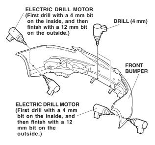
13. Position the left bracket on the inside of the front bumper. Mark the front bumper at the drill point. Align the top of the left bracket with the bead of the front bumper and align the recess at the rear of the left bracket with the flange of the front bumper.
