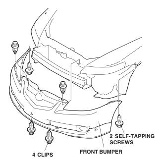
29. Secure the front bumper to the car using four clips, two clips (included in the kit) and two bolts.
