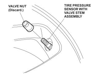
2. Remove and discard the valve stem and the screw from the tire pressure sensor. If the valve stem grommet remained attached to the wheel, remove and discard the grommet before installing the new valve stem.
