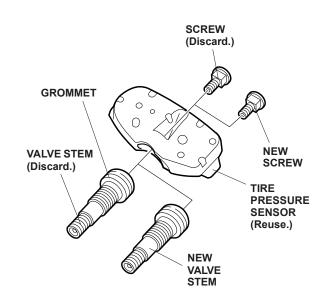
3. Install the new valve stem and screw onto the tire pressure sensor.
