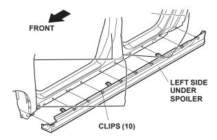
15. Install the three clips (long) and four washers to secure the left side under spoiler. Use one washer on each of the clips that go in the front bracket, and two washers on the clip that goes in the rear bracket.
