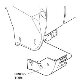
6. Remove 10 clips from the side sill by turning them 45 degrees. Leave the second clip from the front on the vehicle.
