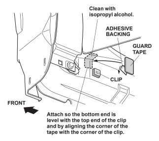
13. Remove the adhesive backing from the guard tape. Attach the guard tape to the vehicle with the bottom end of the guard tape level with the top end of the clip, and align the corner of the tape with the corner of the clip. 14. Position the left side under spoiler on the body, and push the clips into the square holes on the body. Use the palm of your hand to click all 10 clips into place.
