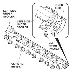
8. Slide nine clips into the slots in the side under spoiler and slide one clip onto the inner trim.
