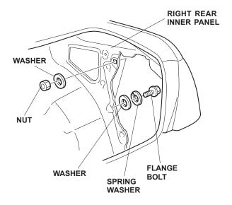
8. Reinstall all removed parts. Check that all clips are installed securely.
