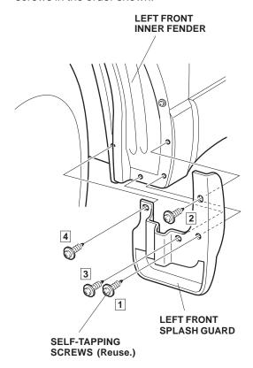
4. Turn the steering wheel all the way clockwise, and repeat steps 2 and 3 to install the right front splash guard.
