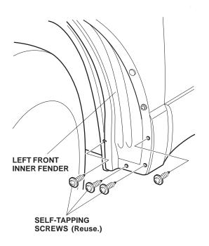
3. Position the left front splash guard on the left front inner fender, and install the four self-tapping screws you removed. Tighten the four self-tapping screws in the order shown.
