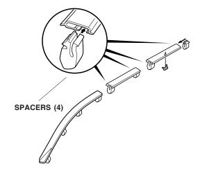
9. Install the cut pieces of left roof molding to the vehicle.
