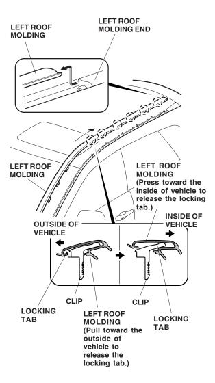
Insert flat-tip screwdrivers alternately between the purple clip and the clip holder as shown. While pulling the purple clip, release the locking tab notch by notch, and remove three purple clips. Work slowly and carefully to remove the purple clips.
