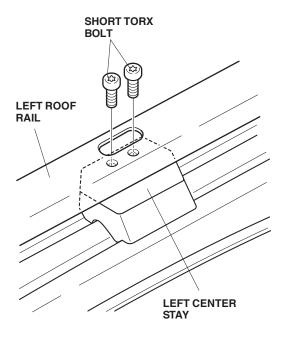
Install two TORX nuts to attach the front stay and rear stays, use a TORX driver to secure the stays to the roof. Torque the four TORX nuts to 7 to 10 N·m (5 to 8 ft·lbs).
