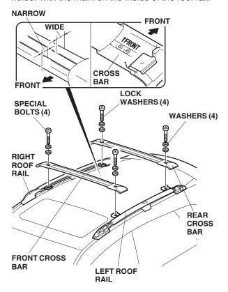
19. Position the cross bars on the holders, and install the special bolts with washers. Tighten the bolts securely.
