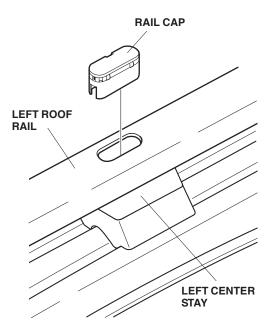
16. Repeat steps 7 thru 15 to install the right roof rail on the right side of the vehicle.
