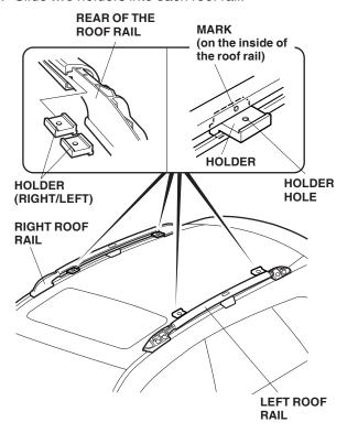
18. Slide each holder back, and align the hole in the holder with the mark on the inside of the roof rail.
