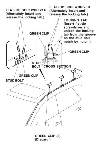
5. Repeat steps 1 thru 4 to remove the roof molding on the right side of the vehicle.
