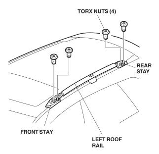
Install the rail cap into the hole in the center of the left roof rail.
