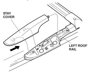
20. After installing, pull the covers back and forth to verify that they are installed securely.
