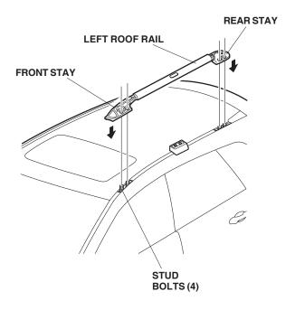
13. At the center stay, install two short TORX bolts through the holes in the left roof rail. Torque the center TORX bolts to 7 to 12 N·m (5 to 7 ft·lbs).
