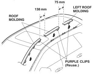
Install the four spacers on the ends of the opieces of the roof molding.
