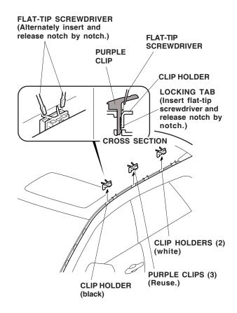
Insert flat-tip screwdrivers alternately between the green clip and the vehicle stud as shown. While pulling the green clip, release the locking tab of the green clip from the groove on the stud notch by notch, and remove the green clip.
