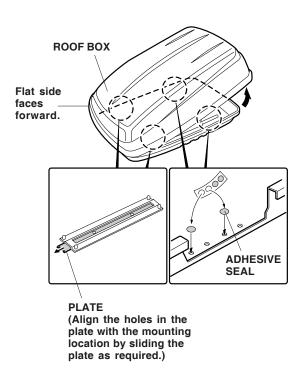
Attach an adhesive seal over each of the four unused mounting holes (two on each side) at the rear of the base of the box. The seals will help prevent water from entering the roof box. 4. Using isopropyl alcohol on a shop towel, clean four brackets B where the small pads will attach. Remove the adhesive backings from the small pads, and attach them to the brackets B.
