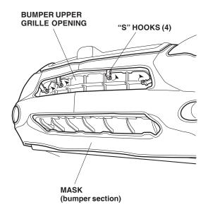
17. Attach the four plastic hooks to the bottom inside edge of the bumper upper grille opening.
