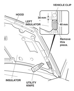
2. Remove the two hood insulator clips. (Do not discard the insulator clips; they can be reinstalled if the mask is removed.)
