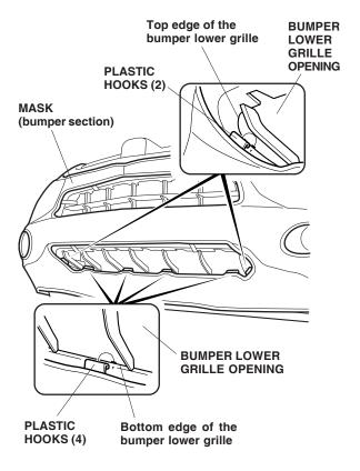
20. Attach the six plastic hooks to the bottom inside edge of the front bumper.
