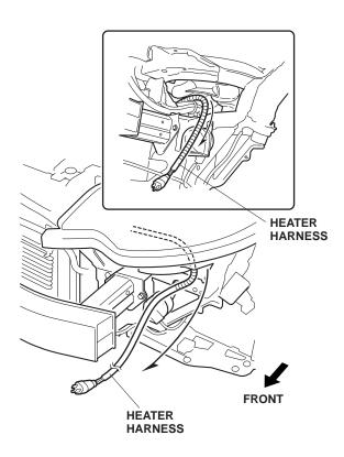
18. Secure the fifth wire tie with clip, that you installed on the heater harness, to the vehicle frame.
