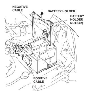
8. Remove the battery cover, battery and battery box.
