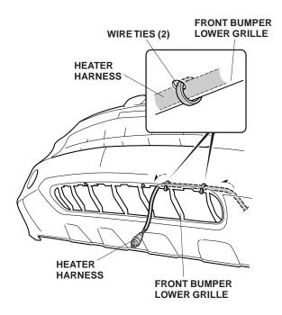
23. Attach the protective cap to the front bumper lower grille, and plug the heater harness connector into the protective cap.
