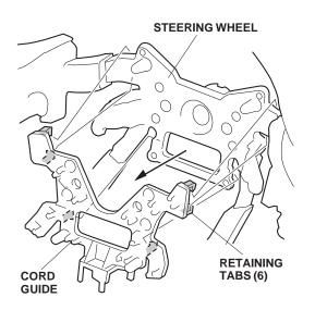
12. Install the cord guide on the new steering wheel.
