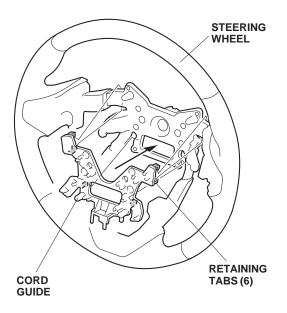
13. Position the switch panel to the steering wheel, and attach the cord to the retaining tabs on the steering wheel.
