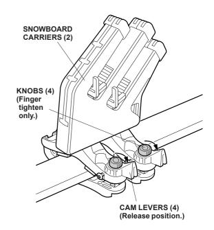
9. Return the four cam levers to the original location (turn clockwise).
