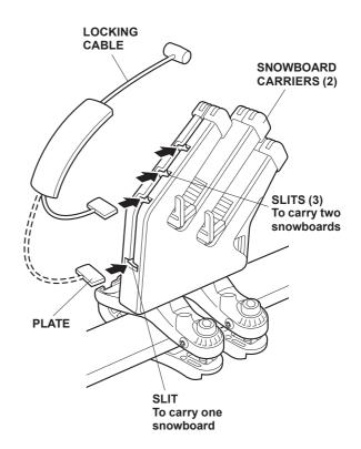
13. After loading the snowboard(s) on the carrier, adjust it (them) with the help of the board supports so that the top edges are level and the boards are as far down in the carrier as possible. To secure the snowboard(s), using the key open the covers insert the locking cable stoppers into the holes of the carrier covers.
