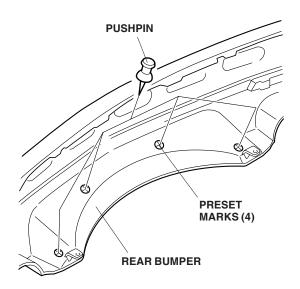
3. While wearing eye protection, drill a hole through each marked location. First drill with a 3 mm drill bit, and finish with a 10 mm drill bit. Remove any burrs from the edges of the holes with a file.
