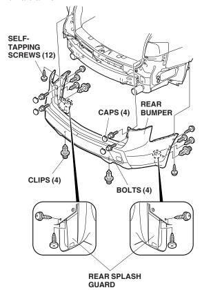
2. On the inside of the rear bumper, locate the four preset marks. Using a push pin, pierce a hole through each mark.
