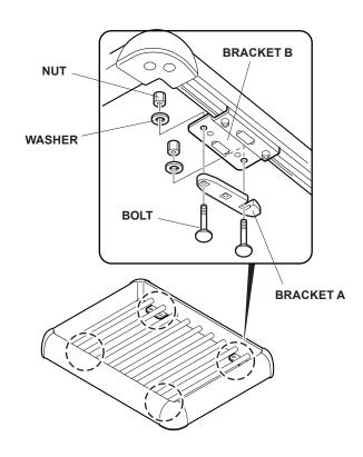
11. Position the roof basket on the roof rack, with the flap from frame A facing forward. Attach the basket to the cross bars by sliding bracket (A) around the crossbar and tightening nuts. Tighten the nuts evenly.
