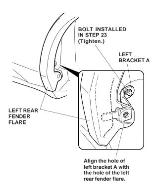
28. Install one 5 x 12 mm self-tapping screw and the expansion clip (removed in step 21) through the holes in the fender flare and the brackets A and B. Do not tighten the screw yet.
