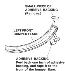
Position the front bumper flare on the front bumper, and align it with the bottom edge of the front bumper. Install two self-tapping screws (5 x 20 mm) through the bumper, but do not tighten them yet.
