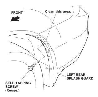
14. Using one alcohol pad provided, thoroughly clean the area where the rear bumper flare will attach.
