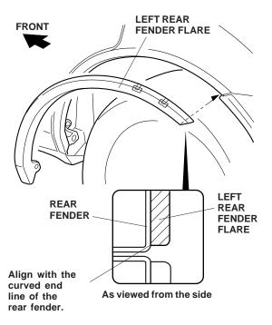
27. Align the hole of left bracket A with the hole of the left rear fender flare and tighten the bolt installed in step 23.
