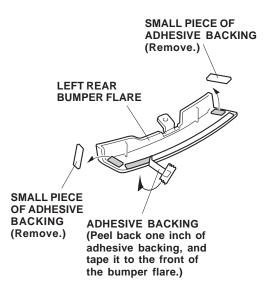
Position the rear bumper flare on the rear bumper, and align it with the top edge of the rear bumper. Install the self-tapping screw through the rear bumper flare, but do not tighten it yet.
