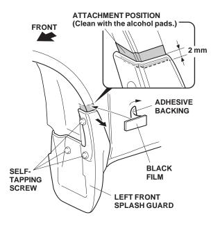
9. Place the left front splash guard in its original position, and tighten the three self-tapping screws.
