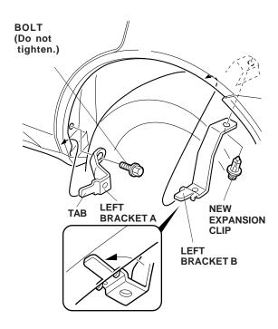
24. Install the left bracket B with the new expansion clip.
