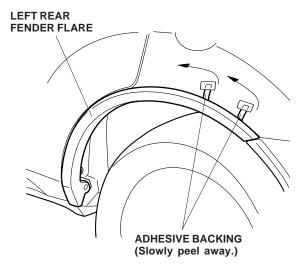
30. Repeat steps 1 through 29 to install the fender flare on the right side of the vehicle.
