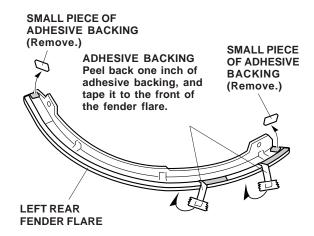
26. Position the rear fender flare on the rear fender as shown.
