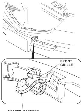
HEATER HARNESS CONNECTOR 16. Secure the heater harness to the vehicle harness using four black wire ties.
