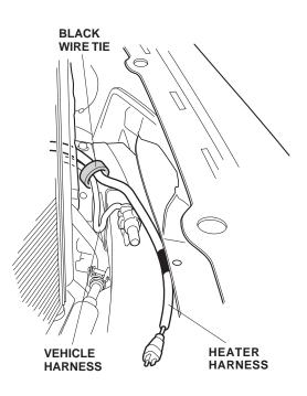
15. Using a black wire tie, secure the heater harness to the front grill as shown. Then attach the protective cap to the grille in the location shown, and install the heater harness connector into the protective cap.
