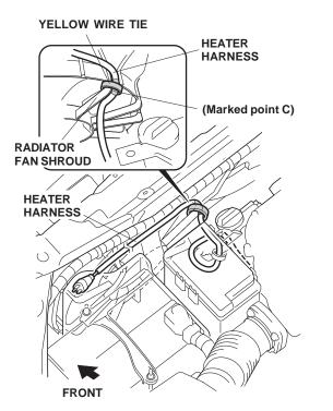
12. Route the heater harness to the left side of the radiator fan along the vehicle harness.
