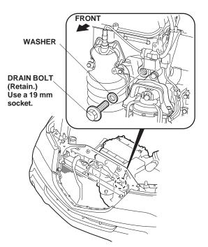
Install the new aluminium washer and the engine block heater into the bolt hole using a 24 mm socket and a torque wrench. Torque the engine block heater to 60 N·m (44 lb-ft).
