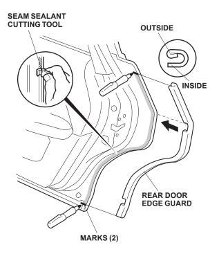
4. Position the cutting edge of the seam sealant cutting tool against the door edge and trim the seam sealant from mark to mark.
