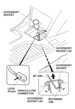
Push the lock tab in and disconnect the vehicle
