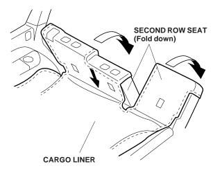
5. Position the cargo liner on the back of the second row seats, and reinstall the headrests.
