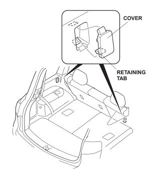
4. Install the cargo cover into the recess in the left rear side panel in the direction shown, then compress the cargo cover, and install it in the right rear side panel.
