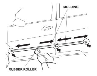
15. Hold the molding firmly against the door with the palm of your hand, particularly at both the edges.
