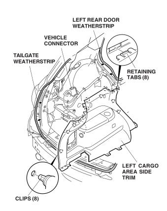
25. Remove the left cargo area side trim (eight clips, eight retaining tabs, and unplug the vehicle connector).
