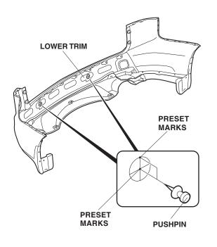
6. While wearing eye protection, drill the lower trim from the painted side at each pierced mark you made. First drill each mark with a 3 mm drill bit, then drill each lower mark with a 26 mm hole saw. Remove any burrs from the edges of the holes with a file.
