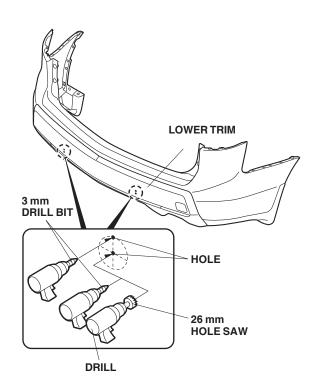
7. On the inside of the rear bumper, locate the two preset marks. Using a pushpin, pierce through the rear bumper at the center and top of the two marks.
