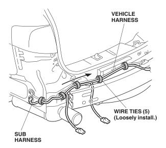
Without Vehicle Harness: Route the subharness along the bumber bean. Loosely install five wire ties with clips to the subharness and insert the clips into the five vehicle panel holes.
