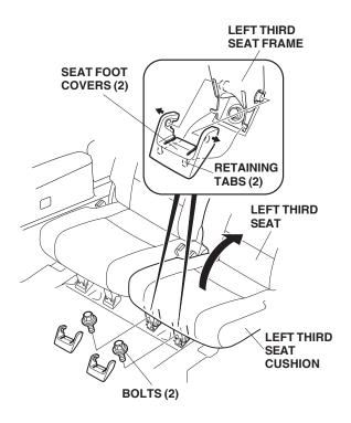
Remove the two bolts that fasten the left third seat to the floor. Raise the left third seat cushion. 19. Remove the four rear bolts that fasten the left third seat to the floor.
