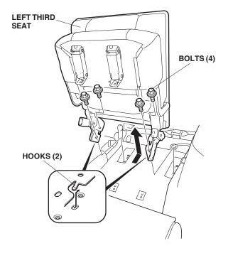
20. Release the two hooks by moving the left third seat rearward, then remove the left third seat.
