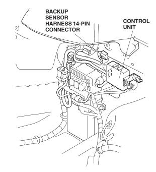
48. Using scissors, cut the EPT sealer as shown. Wrap the small piece of EPT sealer around the backup sensor 4-pin connector, and wrap the large piece of EPT sealer around the 12-pin connector.
