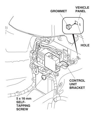
46. Position the control unit bracket on the grommet, and install the 5 x 16 mm self-tapping screw.
