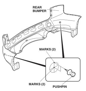
8. While wearing eye protection, drill the rear bumper from the painted side at each pierced mark you made. First drill each mark with a 3 mm drill bit, then drill each lower mark with a 24 mm hole saw. Remove any burrs from the edges of the holes with a file.
