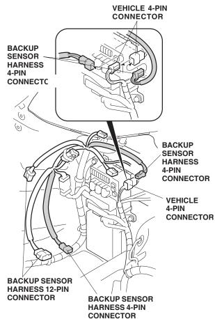
40. Plug the backup sensor harness 12-pin connectors into each other.
