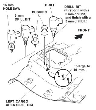
52. While wearing eye protection, drill a 3 mm hole through each of the three pierced points. Then drill the two outer holes with a 5 mm bit. Enlarge the center hole to 16 mm using a hole saw. Remove any burrs from the holes. 53. Route the buzzer harness through the 16 mm hole. With the buzzer switch facing up, install the buzzer with two 4 x 14 mm self-tapping screws with washers.
