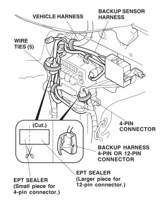
49. Secure the backup sensor harness to the vehicle harness using five wire ties.
