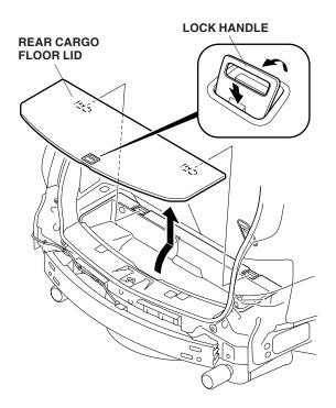
12. Turn the knobs counterclockwise and remove the lid from the rear cargo tray.
