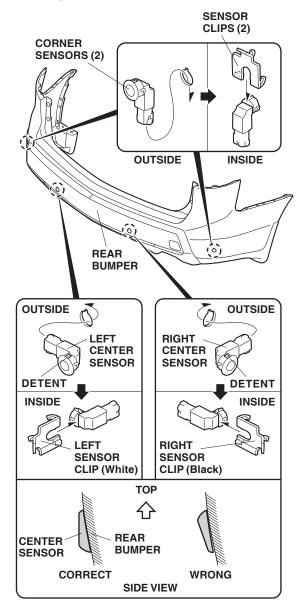
10. Install the right and left center sensors on the rear bumper using the right sensor (black) clip for the right sensor and the left sensor (white) clip for the left sensor.
