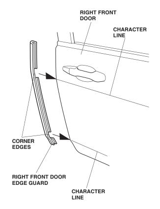
4. Using a felt-tip pen, mark the inside edge of the front door at the upper and lower ends of the right front door edge guard.
