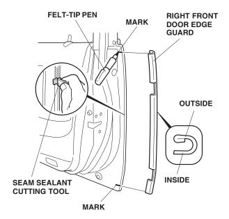
Position the cutting edge of the seam sealant cutting tool against the door edge, and trim the seam sealant between the marks at the top and bottom of the door edge.
