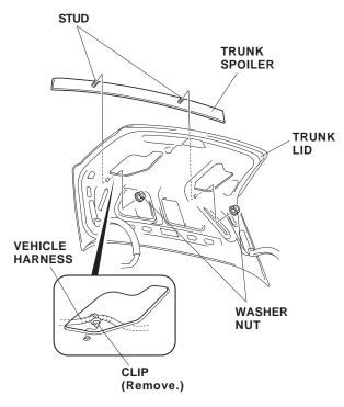
9. Fit the spoiler into position on the trunk lid by inserting the two studs into the holes in the trunk lid. With an assistant holding the trunk lid open, install a flange nut onto the end of each stud, but do not tighten them yet.
