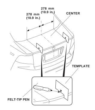
4. Close the trunk lid. Place template B on the trunk lid from edge to edge. Place template A on template B, and line up the marking points. Using a felt-tip pen, mark the trunk at the alignment points as indicated.
