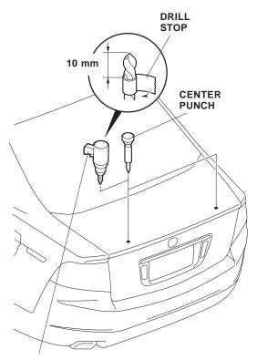
DRILL First drill with a 3 mm drill bit, and finish with an 8 mm drill bit. 6. On the inside of the trunk spoiler, attach a strip of masking tape to the ends of the adhesive backings, and remove 1-1/2 to 2 inches of each adhesive backing. Fold the ends back, and tape them to the front of the spoiler.
