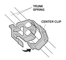
16. With an assistant holding the trunk lid open, remove the left trunk spring from the right trunk hinge bracket using the special tool. Wear gloves to protect your hands, and pull the special tool slowly and carefully toward you.
