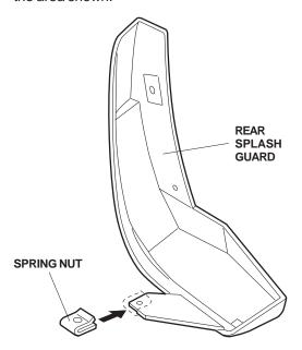
8. Position the left rear splash guard on the left bracket and rear bumper with the spring nut above the bumper. Install the rear splash guard with three self-tapping screws. While holding the splash guard against the bumper to eliminate any gaps, tighten the self-tapping screws.
