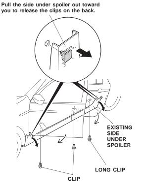
5. Pull the top of the spoiler out, at the front and rear ends, to release the three clips (one at the front and two at the rear).
