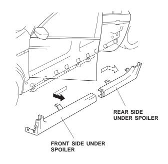
6. Remove the front side under spoiler by sliding it forward and out toward you. Remove the rear side under spoiler by sliding it rearward and out toward you.
