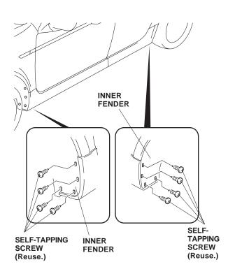
3. Remove the four self-tapping screws that fasten the rear inner fender to the fenderwell.
