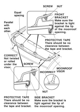
13. Torque the screws to 2 N·m (1.5 lb-ft), alternating between sides
