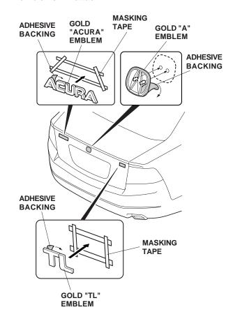
15. Remove the adhesive backings from the gold "A," "ACURA," and "TL" emblems and attach them to the trunk lid so they line up with the tape. Hold the gold emblems firmly against the trunk lid with the palm of your hand for 30 seconds.
