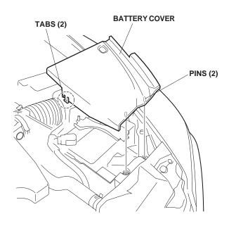
4. Remove the right side cover ( three pins and three tabs).
