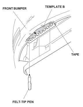
3. Remove the template and center punch the marks you made.
