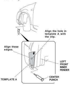
12. While wearing eye protection, drill a 6 mm hole through each center-punched location made in step 11. First drill with a 3 mm drill bit, and then finish with a 6 mm drill bit. Remove all burrs from the edges of the holes with a file. Make sure the front bumper is firmly against the left front inner fender when drilling hole.
