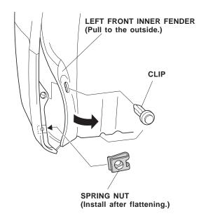
14. Return the left front inner fender to its original position. Get the left bracket, and install the bracket with one clip (reused) and one screw.
