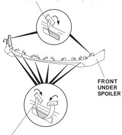
ADHESIVE BACKING WITH TAB (Peel back 1 1/2 - 2 in. of adhesive backing from each side of each adhesive backing and tape each piece to the spoiler using masking tape.)
