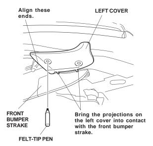
7. Remove the left cover and center punch the marks you made in the bumper.
