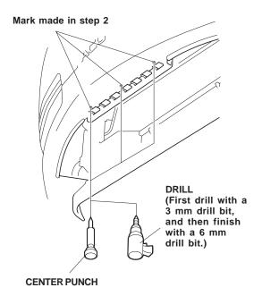
4. While wearing eye protection, drill a 6 mm hole through each marked location. First drill with a 3 mm drill bit, and then finish with a 6 mm drill bit. Remove all burrs from the edges of the holes with a file. 5. Install three spring nuts into the three drilled holes in the bottom of the bumper.
