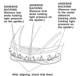
21. Hold the spoiler firmly against the front bumper with the palm of your hand for 30 seconds, particularly at the edges.
