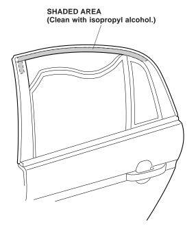
10. Attach a strip of the masking tape to the ends of the three adhesive backings, and remove 50 mm to 80 mm (2 to 3 in.) of adhesive backing. Fold back the ends, and tape the ends to the front of the door visor.
