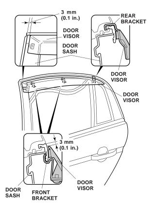
12. Adjust the location of the door visor so that the clearance between the door visor and door sash is 3 mm (0.1 in.) at the front end, and 3 mm (0.1 in.) at the top.
