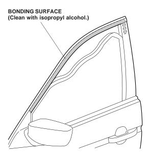
Attach a strip of the masking tape to the ends of the adhesive backings, and remove 50 mm to 80 mm (2 to 3 in.) from the ends. Fold back the ends and tape the ends to the front of the door visor. Note the direction of the adhesive backings.
