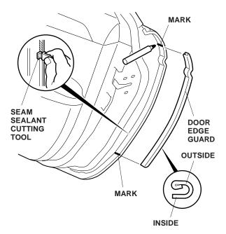
4. Position the cutting edge of the seam sealant cutting tool against the door edge and trim the seam sealant between the marks.
