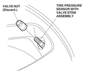
Remove and discard the valve stem and the screw from the tire pressure sensor. If the valve stem grommet remained attached to the wheel, remove and discard the grommet before installing the new valve stem.
