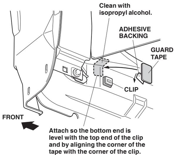
13. Remove the adhesive backing from the guard tape. Attach the guard tape to the vehicle with the bottom end of the guard tape level with the top end of the clip, and align the corner of the tape with the corner of the clip.
