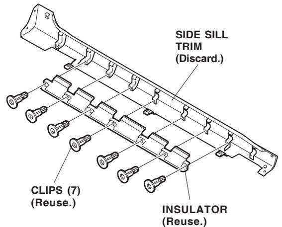
11. Install the insulator to the left side under spoiler with the seven clips.
