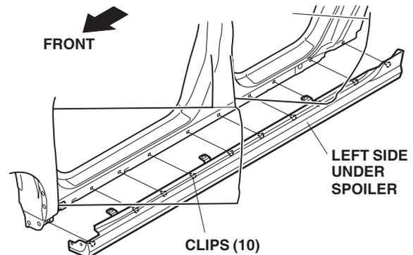
15. Install the three clips (long) and four washers to secure the left side under spoiler. Use one washer on each of the clips that go in the front bracket, and two washers on the clip that goes in the rear bracket.
