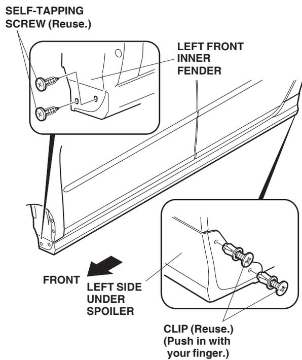
17. Reinstall the two clips you removed in step 2 by pushing them in with your finger.
