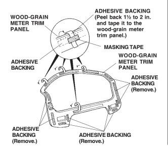
Apply pressure against the wood-grain meter trim panel, carefully remove the four adhesive backings you taped to the wood-grain meter trim panel. Continue to apply pressure to the wood-grain meter trim panel with the palm of your hand for at least 30 seconds.
