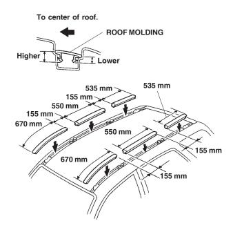
6. Position the front and rear roof racks on the roof by aligning the holes with the studs of the roof, and install the Torx nuts through the holes onto the studs. Using a T-30 Torx driver, torque the nuts to 7 to 10 N•m (5 to 8 lb-ft).
