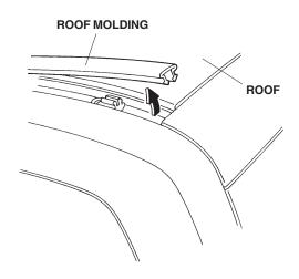
3. If a clip is attached to the roof molding after removing the roof molding, remove the clip and reposition it on the roof.
