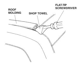
2. Remove the roof moldings by carefully pulling them upward.
