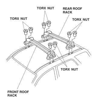
7. Align the tab on the roof rack cover with the groove in the roof rack, and install the roof rack covers.
