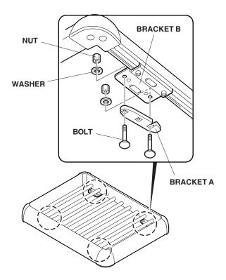
11. Position the roof basket on the roof rack, with the flap from frame A facing forward. Attach the basket to the cross bars by sliding bracket (A) around the crossbar and tightening nuts. Tighten the nuts evenly.
