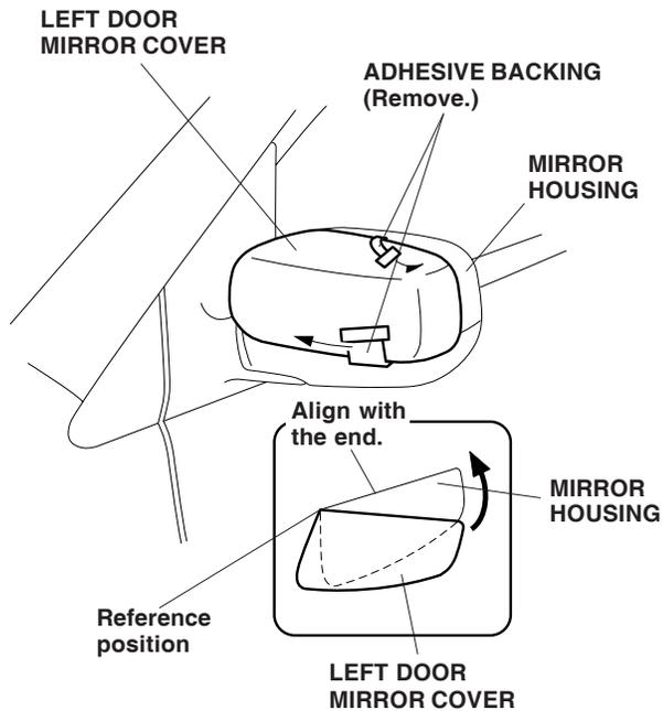
4. Using the palm of your hand firmly press the mirror cover against the mirror for 30 seconds, particularly at the edges.
