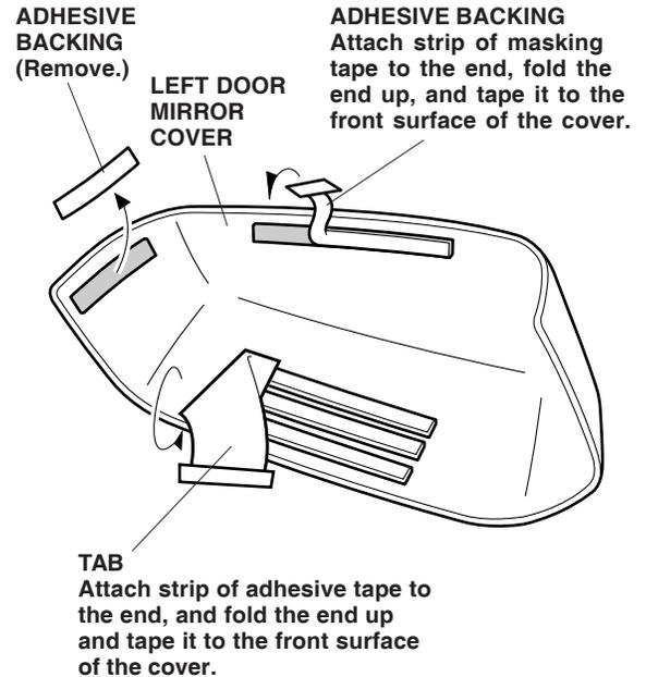
2. Attach strips of masking tape to the ends of the upper adhesive backing and center tab. Fold those ends up, and temporarily tape them to the surface of the door mirror cover. Remove the remaining adhesive backings.
