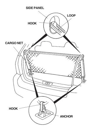
Put these instructions and the remaining two hooks (if necessary) in the glove box for your customer.
