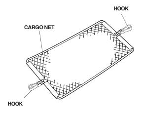
3. Fold the cargo net in half, attach the hooks to the anchors in the floor, and attach the loops to the hooks on the side panel.
