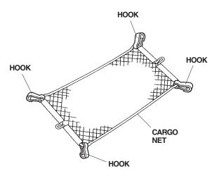
6. Attach the hooks to the anchors in the cargo area.
