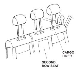
5. Install the cargo liner over the second row seats, and reinstall the headrests.
