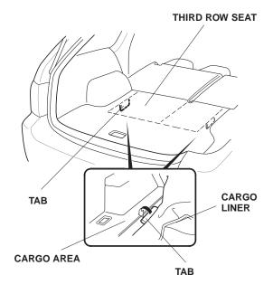
Open the floor storage compartment, and fit the pocket of the cargo liner around the storage compartment cover.
