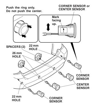
14. Install the two center sensors into the 26 mm holes. Install the two center sensors by embedding them, as shown, in the two 26 mm holes you just made. Secure the center sensors with one spacer for each sensor. Push only the ring on the sensor circumference. Pushing the center of the sensor could damage the sensor.
