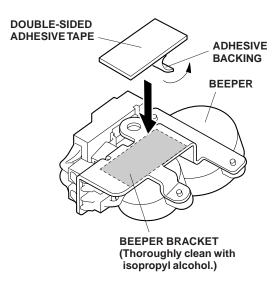
44. Using isopropyl alcohol on a shop towel, clean the inside rear panel where the beeper will attach. Remove the adhesive backing from the double-sided tape on the beeper, and attach the beeper to the inside rear panel. You must have 5 mm of clearance between the 5-pin connector and the edge of the inside rear panel. Hold the beeper in place for 30 seconds.
