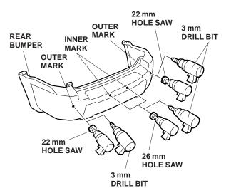
13. Install the two corner sensors by embedding them, as shown, in the two 22 mm holes you just made. Push only the ring at the sensor circumference. Pushing the center of the sensor could damage the sensor.
