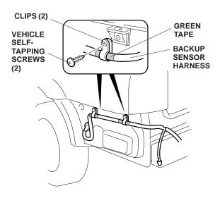
34. Attach the four wire ties with clip to the backup sensor harness where the green tape is located, then push the clips into the holes in the bumper beam and body frame. If a trailer hitch is installed, cut the clip off the wire tie with clip, align the green tapes on the trailer hitch and backup sensor harnesses, and then secure the harnesses with the wire tie.
