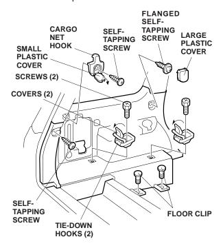
28. Remove the large plastic cover, and remove the flanged self-tapping screw concealed under the cover. Pry out the small plastic cover with a trim tool, and remove the cargo net hook (one self-tapping screw). Remove the self-tapping screw.
