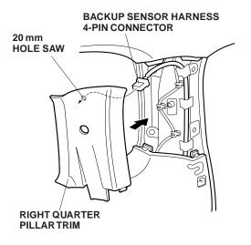
58. Plug the backup sensor harness 4-pin connector into the switch, then install the switch into the hole in the right quarter pillar trim, in the direction shown.
