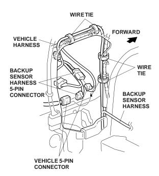
38. Unplug the vehicle 5-pin connectors, and plug them into the backup sensor harness 5-pin connectors.
