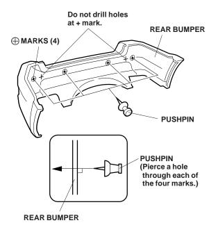
12. While wearing eye protection, drill a 22 mm hole through each of the two outer marks, and a 26 mm hole through each of the inner marks. Remove any burrs from the edges of the holes. First drill with a 3 mm drill bit, and then finish with a 22 mm hole saw or a 26 mm hole saw.
