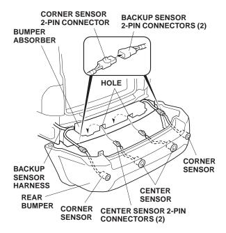
60. Connect the two outer backup sensor harness 2-pin connectors to the 2-pin connectors from the corner sensors. Reinstall the rear bumper. Check that all clips and retaining tabs are installed securely.
