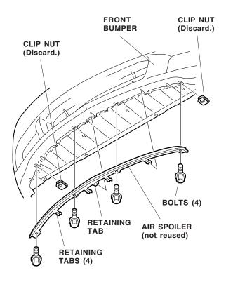
2. Remove the two bolts and five clips from the bottom of the front bumper.
