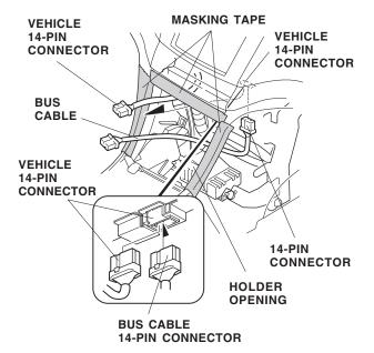
8. Wrap one wire tie with clip around the bus cable, and push the wire tie with clip into the hole in the vehicle frame.
