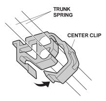
16. With an assistant holding the trunk lid open, remove the left trunk spring from the right trunk hinge bracket using the special tool. Wear gloves to protect your hands, and pull the special tool slowly and carefully toward you.
