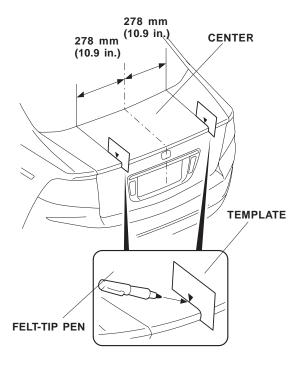
4. Close the trunk lid. Place template B on the trunk lid from edge to edge. Place template A on template B, and line up the marking points. Using a felt-tip pen, mark the trunk at the alignment points as indicated.
