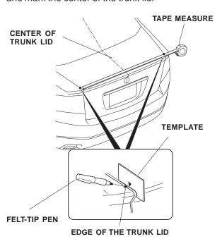
Measure 10.9 in. (278 mm) outboard from the center and mark the trunk lid on each side.
