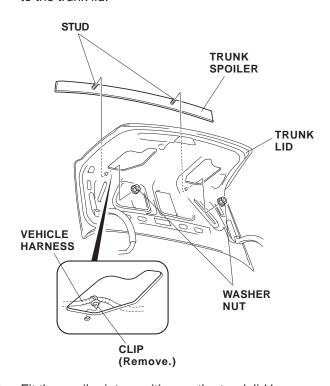
Fit the spoiler into position on the trunk lid by inserting the two studs into the holes in the trunk lid. With an assistant holding the trunk lid open, install a flange nut onto the end of each stud, but do not tighten them yet. 10. When the trunk spoiler is aligned properly with the trunk lid, carefully remove the adhesive backing on each side. Hold the spoiler firmly against the trunk lid with the palm of your hand.
