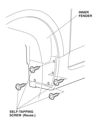
3. Position the left front splash guard on the left inner fender, with the tang from the splash guard around the side sill. Reinstall the four self-tapping screws.
