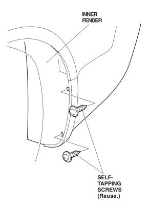
6. Position the left bracket on the inner fender, and reinstall the two self-tapping screws.
